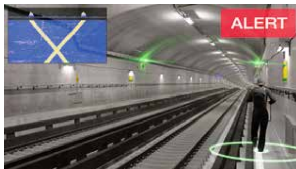
Fig 3. DAS can be used to detect people on the track, triggering an alert to warn of trespassing and potential criminal activity.
